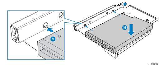
Figure 20. Installing a Floppy Drive into the Slimline Carrier
